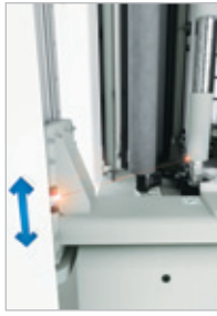
Automatic laser core guiding 08
