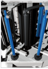
Tenzomat III rewinding tension control 11
